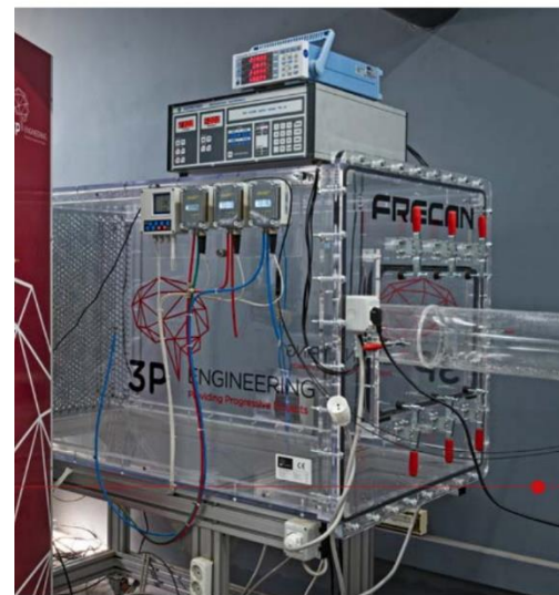
On the right: The Airflow Test Bench of 3P Engineering: tests on Frecan products
